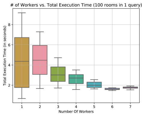
Fig. 7. Execution times for large sets of data in single queries with varying number of workers
